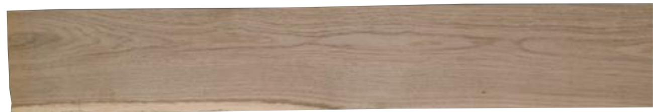
**This oak board includes an area of sapwood in the bottom left corner. Sapwood needs to be excluded if oak is to be used as external cladding or other joinery product where the timber will get wet for extended periods. Sapwood should also be excluded in sweet chestnut if it is to be used out-of-doors.**
