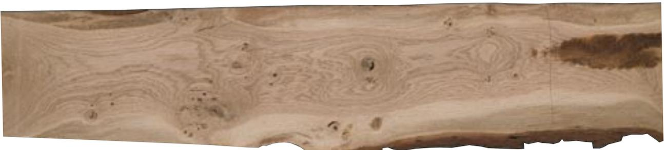
This grade 2 oak board has been measured to exclude the area of bark on the right - the area measured-out has been marked on the board using a vertical line.
